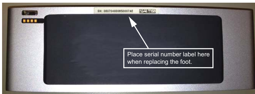
SoundLink Mini II Serial Number Placement (when replacing the foot)
