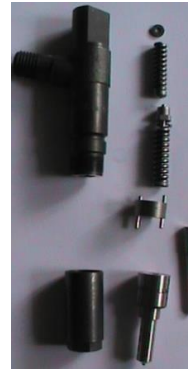
Figure 11. Structure of D1703-M-DI engine nozzle. 1. Injector body, 2. Locking nut, 3. Body longitudinal fuel pipe, 4. High pressure hose connection, 5. Oil return line connection, 6. Injector body, 7. Adjusting gasket, 8. 1st stage spring, 9. Spring stop plate, 10. Guide tube, 11. Adjusting pad, 12. 2nd stage spring, 13. Push rod, 14. Intermediate connecting pin, 15. Setting base maximum injector lift stroke position, 16. Locating pin, 17. Nozzle body, 18. High pressure chamber, 19. Injector.
