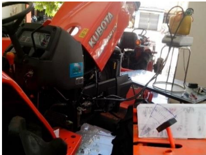
Figure 24. Measuring fuel consumption of Kubota D1703-M-DI engine.
