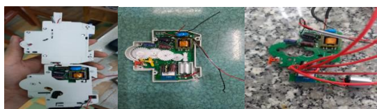
Figure 7. Construction and simulation of control circuit signals for switchgear
