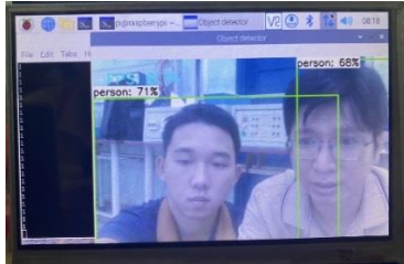
Figure 4. Object detection with TensorFlow Lite model.
