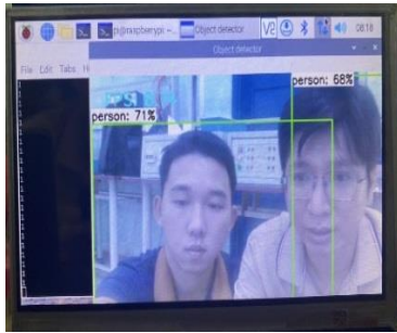
Figure 4. Object detection with TensorFlow Lite model.
