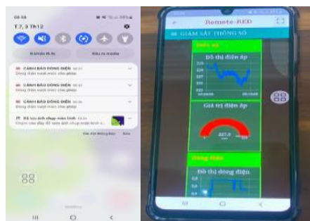
In addition to computer monitoring and control, the system also allows phone interface and function synchronization as shown in Figure 15.
