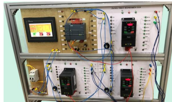
Figure 9. Pump station monitoring and control model based on Modbus RTU network.
