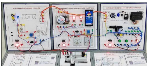
Figure 6. Practicing wiring of key and Start/Stop button starting systems on the model.
