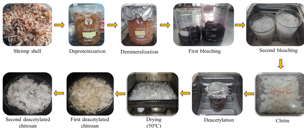
Figure 1. Chitosan preparation using shrimp shells
