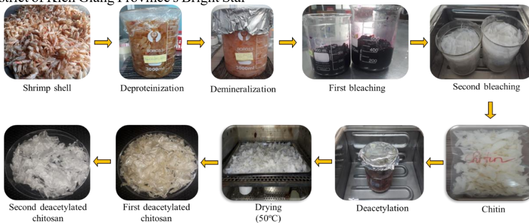
Figure 1. Chitosan preparation using shrimp shells
