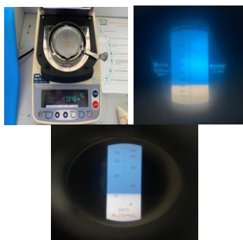
Figure 1 Measurement of moisture, Brix and alcohol content of sample
