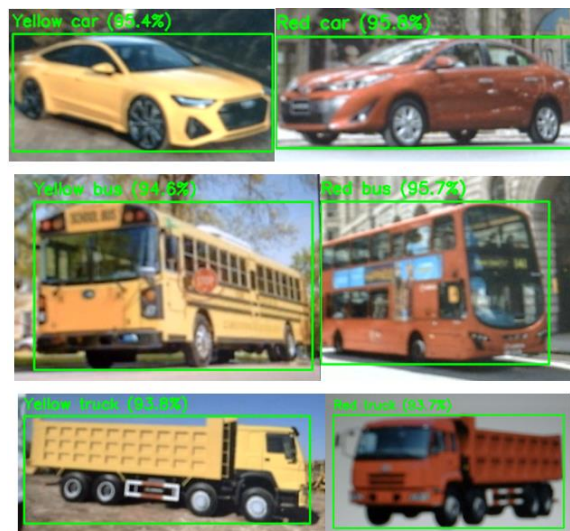
Figure 12. Vehicle and color recognition using YOLO and HSV
