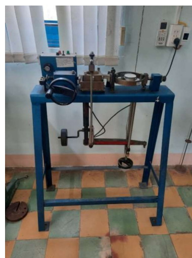
Figure 4. The two-speed soil shearing machine.
