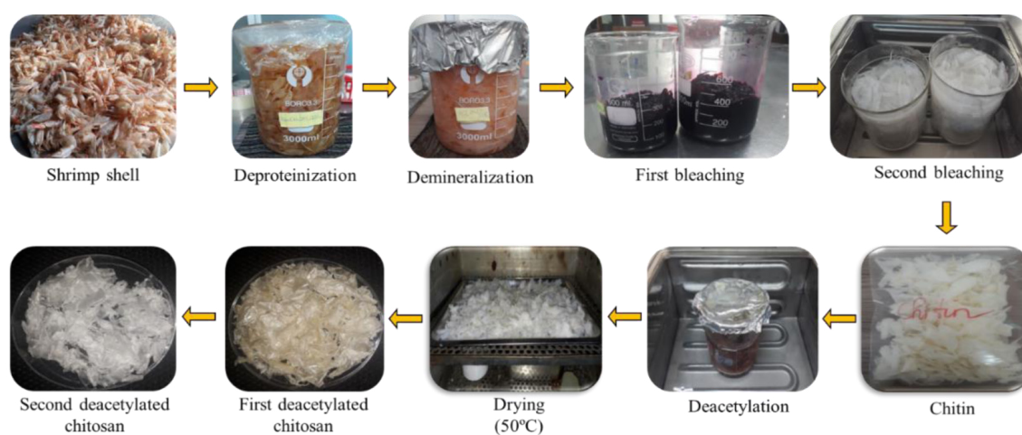
Figure 1. Chitosan preparation using shrimp shells.
