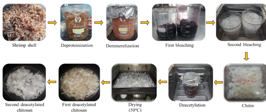
Figure 1. Chitosan preparation using shrimp shells.
