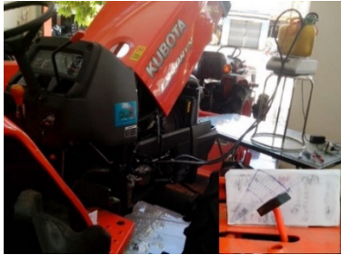
Figure 24. Measuring fuel consumption of Kubota D1703-M-DI engine.
