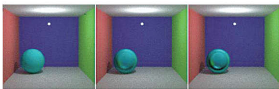
Figure 5. Rendering images from left to right of different cases of spherical reflection: uniform scattering, directional scattering, mirror reflection
