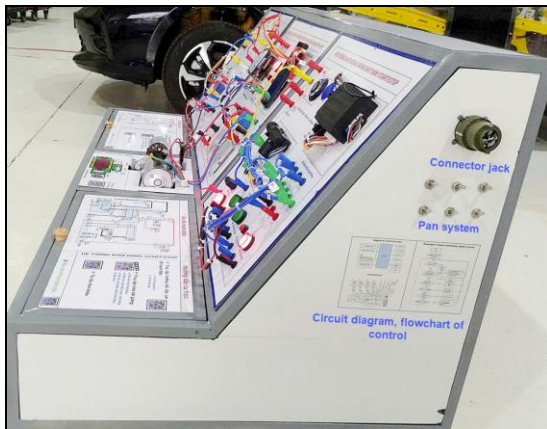
Figure 2. Side view of the smart starting system model for remote automobile control via smartphone.
